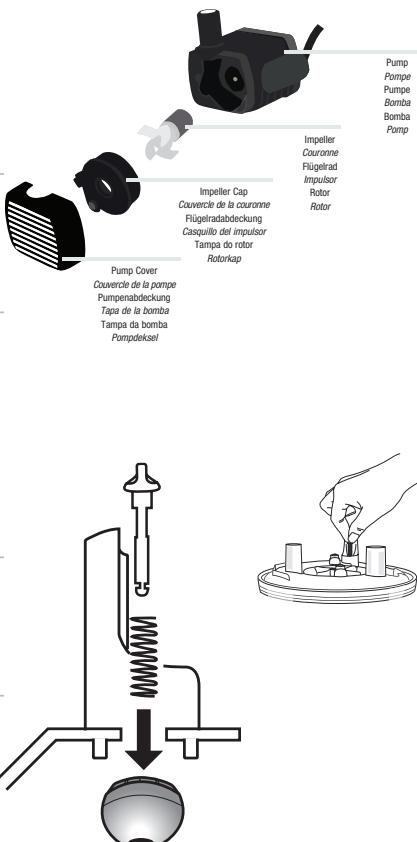
To reassemble valve assembly, place spring on stem. Slide stem with spring through the valve opening. Attach blue rubber cap to stem.
