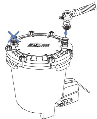
6. Position the hose opening in an appropriate drain basin.
