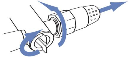
4. Attach one end of a flexible 5/8 in.(1.58cm) diameter hose (not supplied) to the Purge valve, and position the other end in an appropriate basin or discharge drain. If not using the Fluval ribbed hosing it may be necessary to use a clamp to secure the hose in place.
