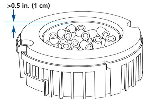
6. Stack the baskets, carefully aligning them, so that all shapes match. Reinsert the T-handles into their vertical slots, and replace the baskets in the filter canister. The foam in the upper basket should be just about even with the top edge of the canister (*the output tube, which is affixed to the inside of the canister, will be protruding slightly*).
