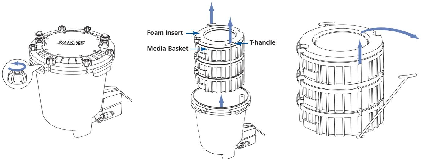
4. Rinse the media baskets and foam inserts under running tap water to remove any dust particles.
