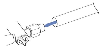
5. First, turn the Purge valve to the open (horizontal) position by turning it counter-clockwise. Then disconnect the IN valve: press its release button, and lift it from the filter lid. It is a good idea to have a cloth handy as some water will escape when removing the AquaStop Valve.
