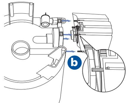
4. Clean the impeller and the impeller well thoroughly by rinsing with clear running water.
