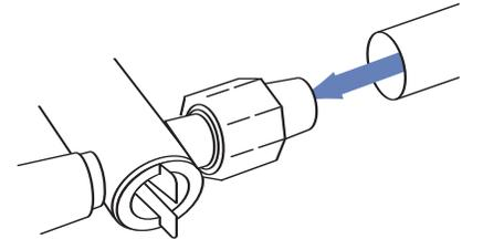
5. a. First, turn the Purge valve to the open (horizontal) position (rotate it counter-clockwise).
