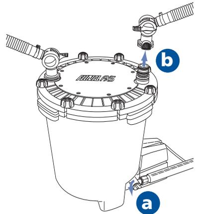
6. Water will immediately begin to drain from the canister.
